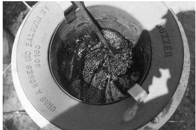
Fig. 3 Vitrified paint debris being remelted and stirred in pot-type furnace to immobilize lead
